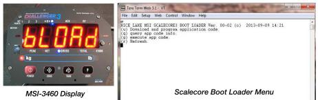
Figure 8-3. Access Bootloader Within Scalecore
