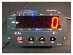
Figure 8-7. Normal Weighing Mode
