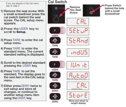
Figure 5-9. Weight Standard Setup
