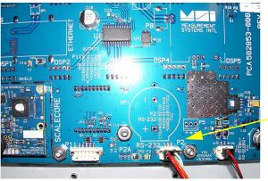
Figure 8-1. Connecting Interface Cable
