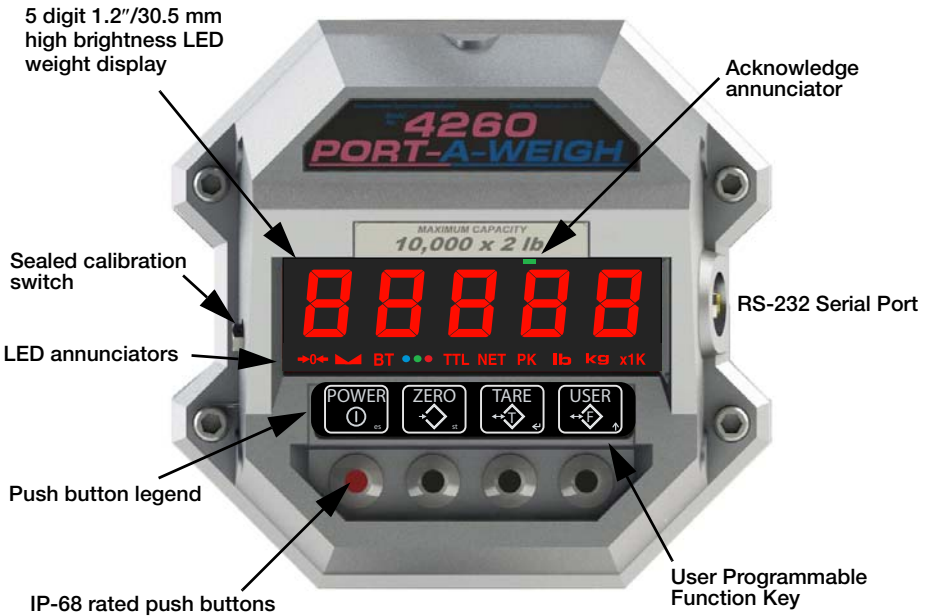
Figure 1-1 MSI-4260 Front Panel
