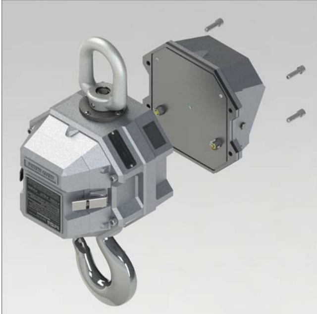
Figure 1-5 Remove Front Casting
